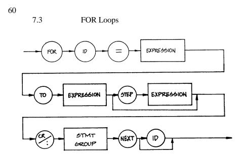
On each iteration through the loop, the index is incremented by the value of the step expression. If the step expression is omitted, the index is incremented a value of 1 (the default value). The general form of a FOR loop header is shown below.
