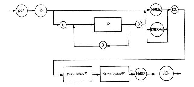
The executable block can contain any CB-80 executable statements. However, function definitions cannot be nested. A multiple line function cannot contain another multiple line or a single line function definition. In addition, recursive references are not supported.
