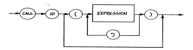
CALL statements pass actual parameters to a multiple line function and then execute the function. The address of the statement following the CALL statement is saved on a Last-In-First Out (LIFO) stack. So, statement execution can continue with (or return to) the statement following the CALL. A RETURN statement or a FEND statement returns execution to the statement following the CALL.
