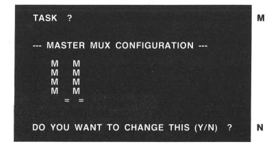
The MUX table is used to specify what is connected to the master multiplexer. It is usually set to assume that all the slots have MUX on them. This allows it to work correctly on systems that are only using a host multiplexer.
